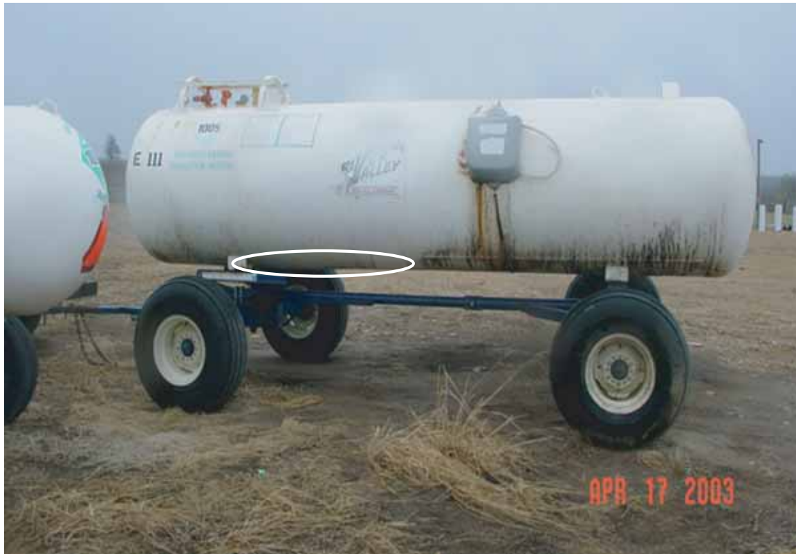
Figure 1. Accident nurse tank with shell fracture area circled.
