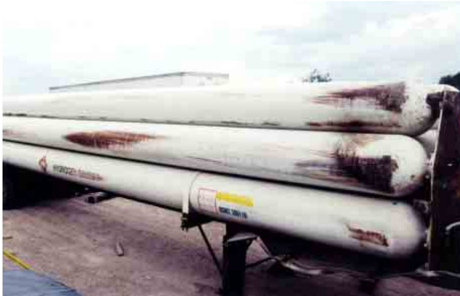
Figure 5. Scrapes on the outboard sides of cylinders on the accident semitrailer.
