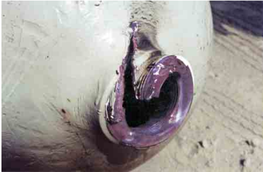
Figure 7. Cylinder 3's forward end, which has an overstress fracture on its shoulder and a spiral crack from the fracture surface into the head of cylinder.
