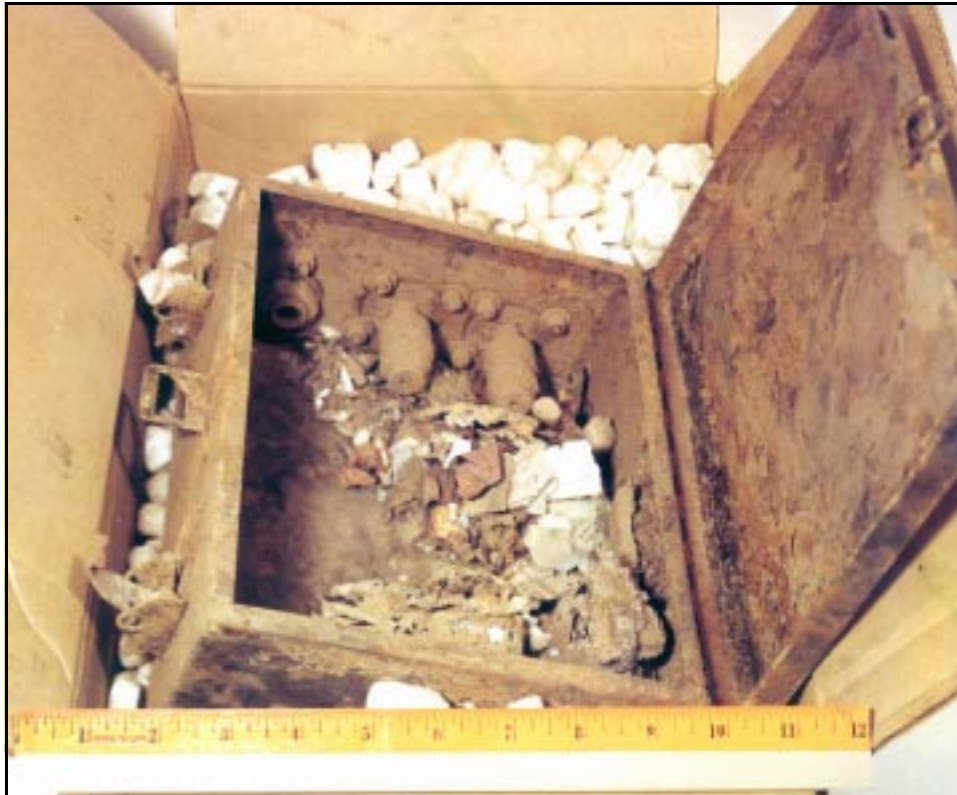
Figure 9. The event recorder from UP 3616, train NP-01's lead locomotive
