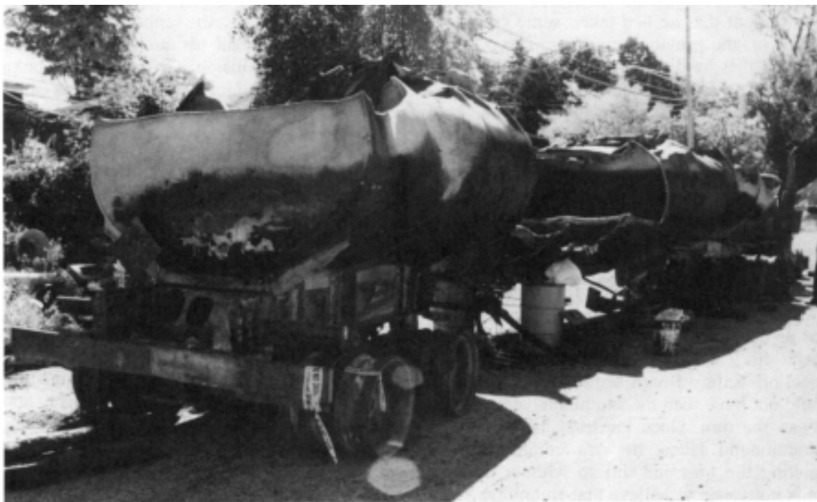
Figure 6.—Melted tanker truck.
