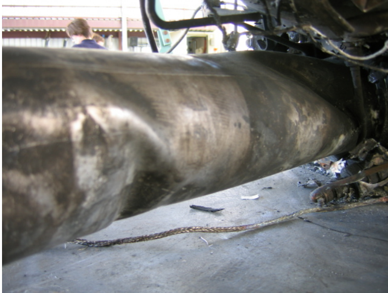
Figure 20. Turbomeca picture of linking tube - torsional twist
