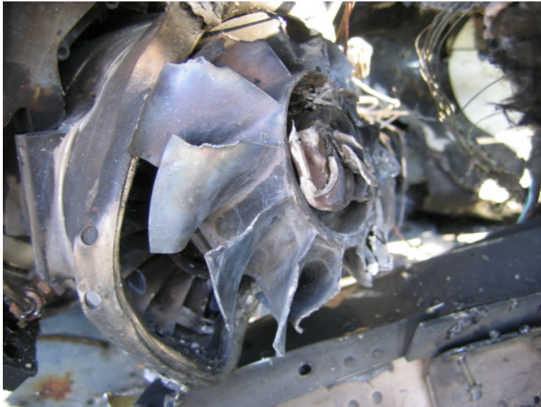
Figure 18. Turbomeca picture of axial rotor and nose bullet detailing bending and smearing opposite to the direction of rotation
