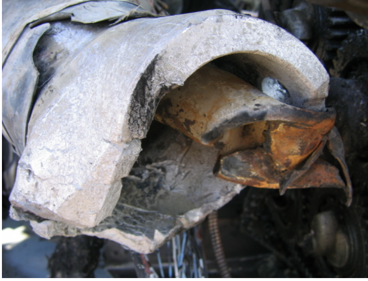
Figure 19. Turbomeca picture of coupling tube and transmission shaft - showing torsional twist
