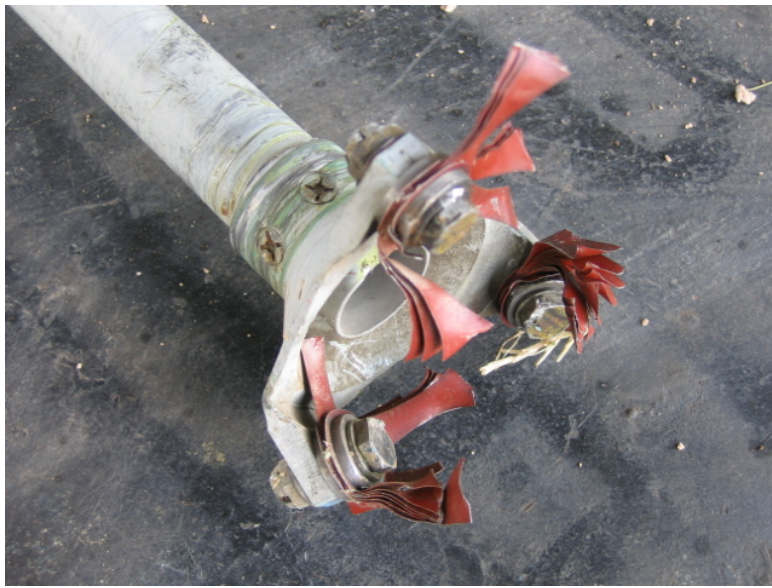
Figure 11. Turbomeca picture of short shaft - rotational scarring
