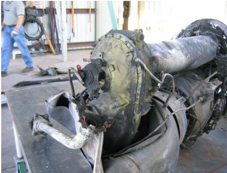
Figure 20. Turbomeca picture of flange at the rear of the turbine reduction gear and short shaft
