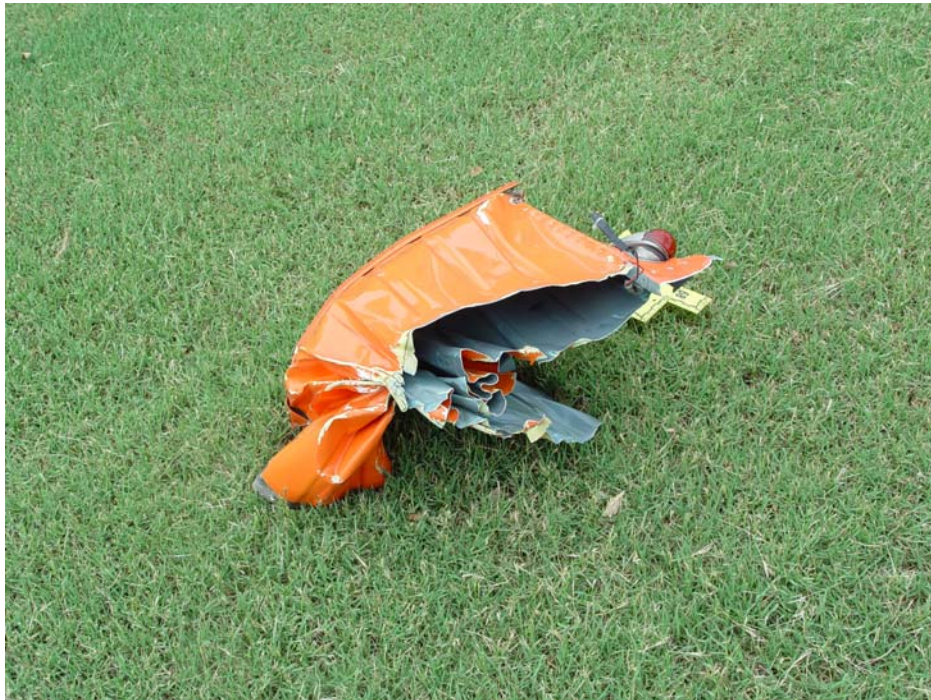
Figure 14. Ch 3-accordion left horizontal stabilizer piece
