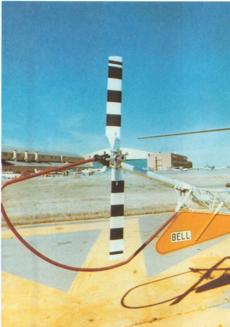
FIGURE 12. Helicopter tail rotor with black and white asymmetrical paint scheme, U.S. Army TB-746-93-2.
