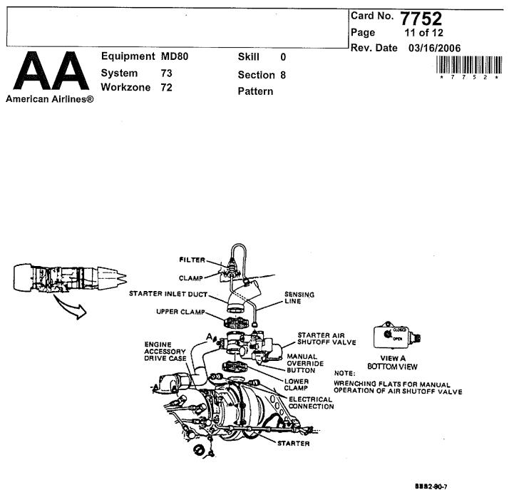
Starter Air Shutoff Valve - Installation Figure 4:
