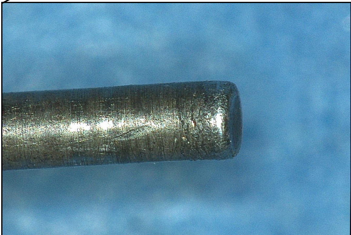
Figure 3--The bent push button pin with an enlargement showing the deformed and dented end.
