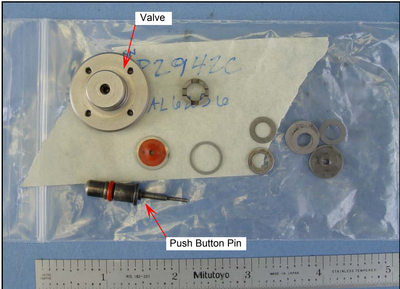
Figure 1--An overall view of the as-recieved components from the air interrupt solenoid valve, s/n P2942C. The bent push button pin is noted.
