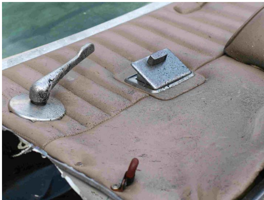
Figure 6 – Deposits on Cabin Door
