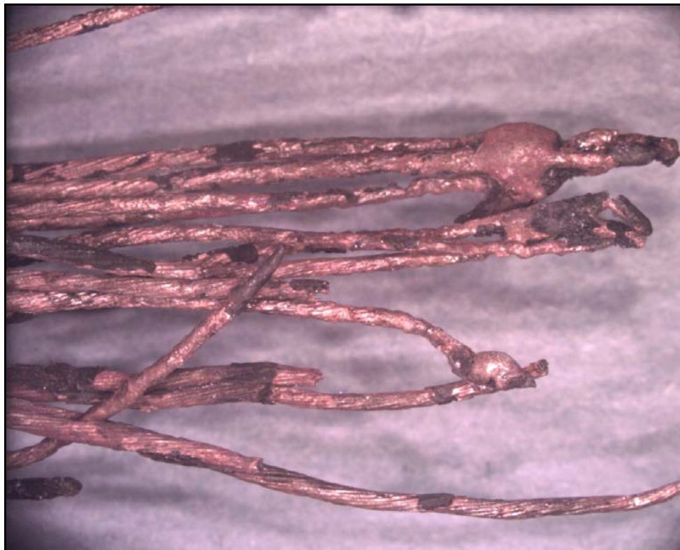
Figure 2. Beading on end of wire bundle.
