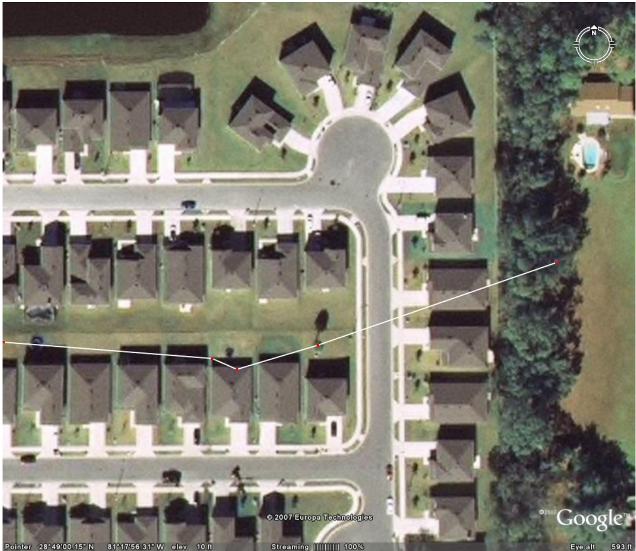
Figure 6. Debris Track (Points are 1 st Impact, Palm Tree, Wing Box, Empennage and Propeller). Cumulative linear distances are 0, 270, 357, 386 and 608 feet respectively; Incremental distances are 0, 270, 87, 29, and 379 feet respectively.
