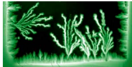
Figure 32 Magneto-optical image of magnetic flux avalanches penetrating into a \text{MgB}_2 film at 5 K (Image courtesy of T.H. Johansen, University of Oslo).
