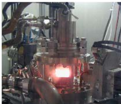
Figure 40 In situ X-ray study of (In,Ga)N growth in the high-temperature, reactive environment of metal-organic chemical vapor deposition.
