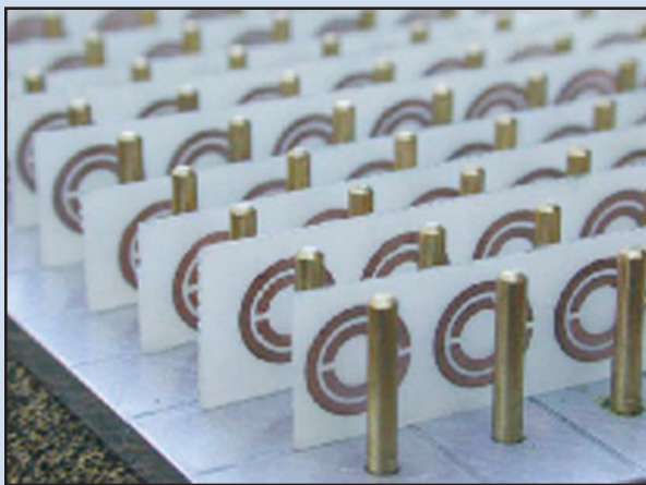
FIGURE 1. Negative-Index Material (NIM) that operates at microwave frequencies.
