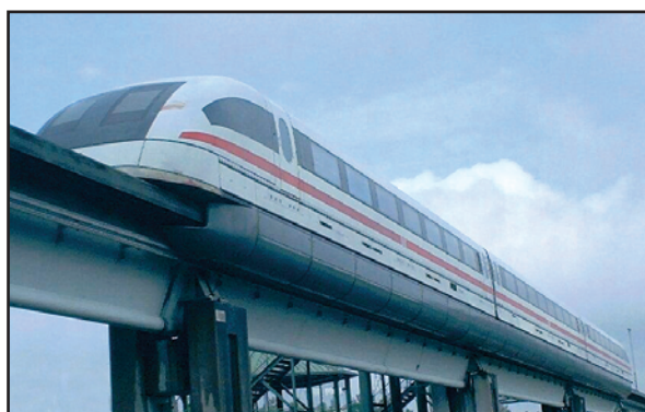
FIGURE 3.11. Magnetic levitation of high-speed trains using low-temperature superconductors. Creating new high-temperature superconducting materials with current-carrying and processing characteristics far superior to those achievable today would provide the means for a complete sea change in transportation systems and in energy transmission.
