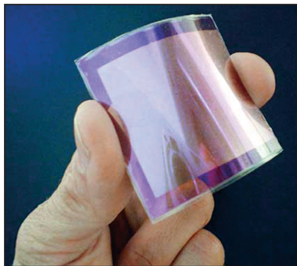
FIGURE 3.2. A flexible solar cell, the active region of which is made from polymeric soft-matter organic materials. Significant advances in materials design and synthesis will be required to achieve needed power-conversion efficiencies.
