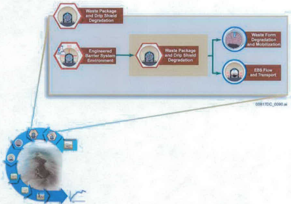
Figure 6.3.5-2. Information Flow Diagram for Waste Package and Drip Shield Degradation
