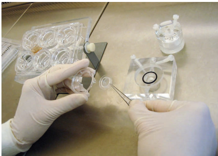
Now on the air. Human cells grown on ready-made culture inserts are placed in a horizontal diffusion chamber to test the effects of airborne chemicals.
