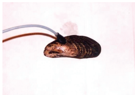
Figure 6. Atlantic ribbed mussels were used as the bioindicator organism for New Bedford Harbor. Their heart rate was monitored using an infrared heart rate monitor attached to the surface of the mussel's shell. Photograph courtesy of Ross Sanger, University of Plymouth.
