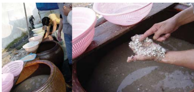
Figure 6. Plastic reprocessing by gravitational separation into ceramic jugs with brine.
