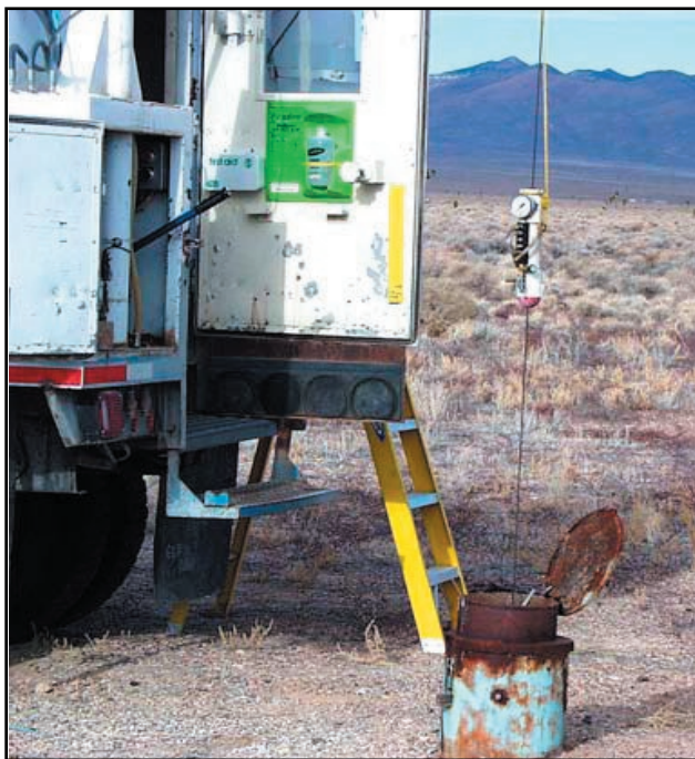
Taking a water sample from an NTS non-potable groundwater monitoring well (photo by Terrence Sonnenburg, May 2002)
