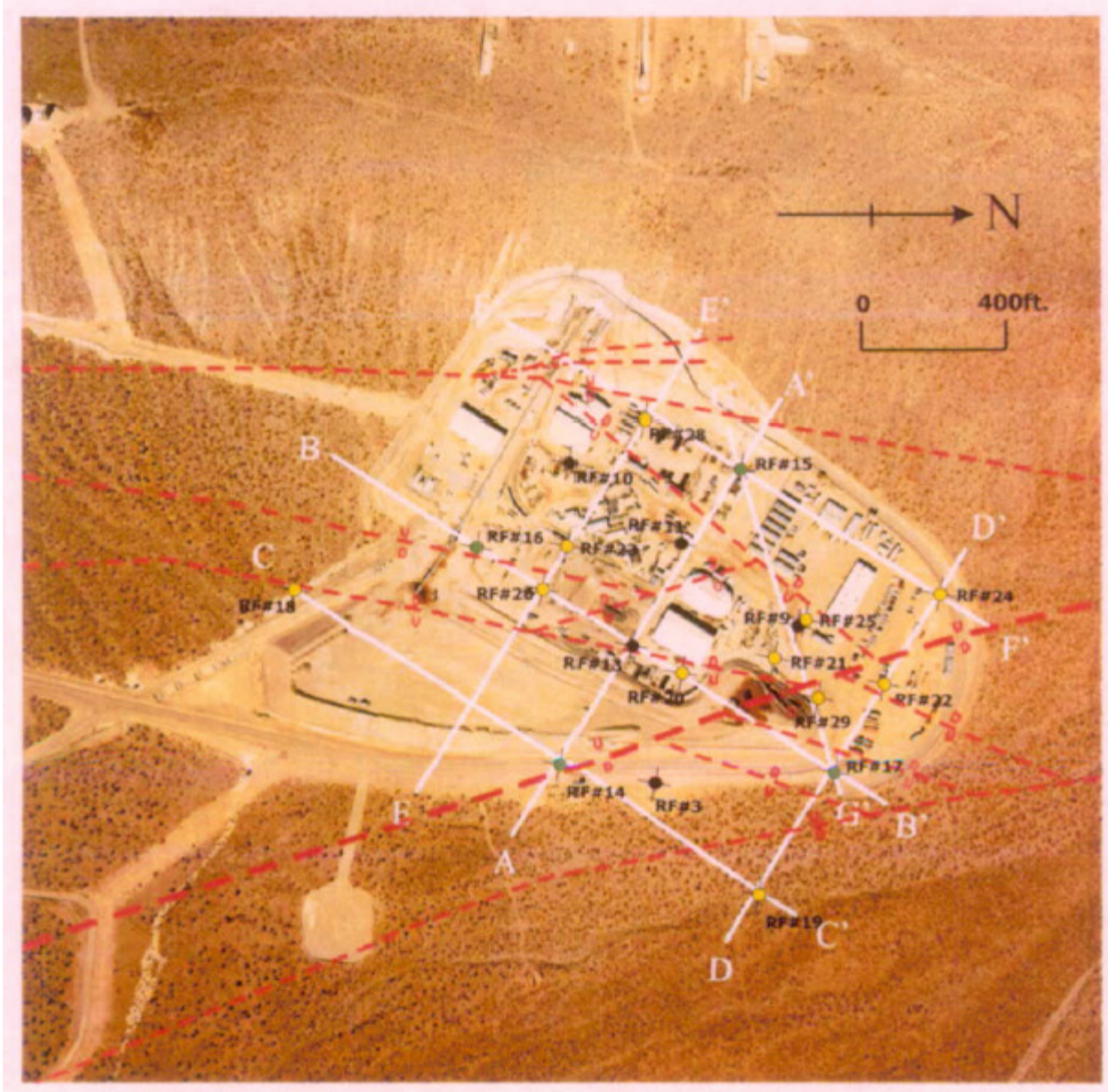
Figure 6-7. Locations of Soil Exploration in the surface facilities area (only pre-2005 borings shown). Cross-Sections shown in Figure 6-4, Figure 6-5, and Figure 7-1.
