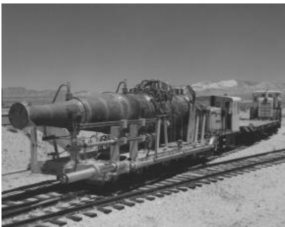
Nuclear ramjet engine on its test bed facility, a railroad flatcar. Source: REECO, Bechtel Nevada.
