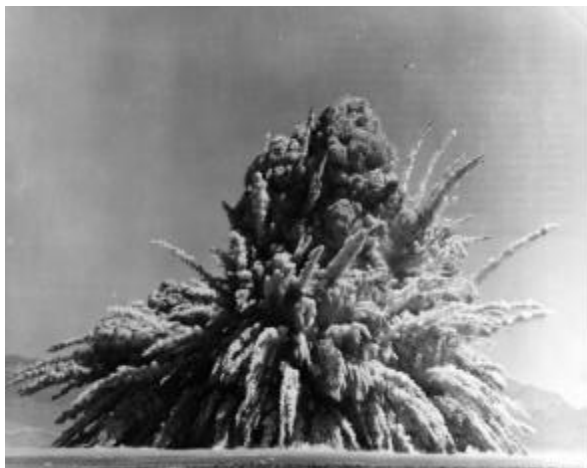
Plumes of sand and dust formed by boulders and clumps of gravel ejected from the desert by the July 6, 1962, Sedan Plowshare test. Source: REECO, Bechtel Nevada.
