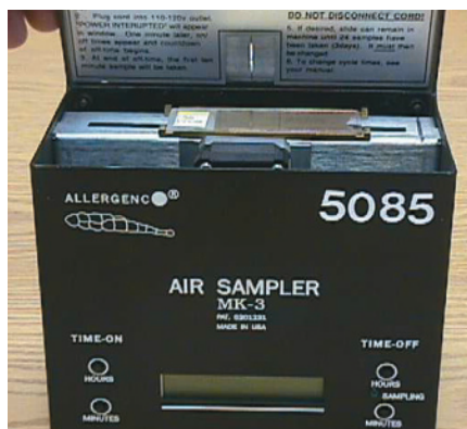
Figure 1. Photograph of the Allergenco MK-3 air sampler (Allergenco/Blewstone Press, San Antonio, TX). Airborne particulates drawn through a small opening (1.1 × 14.5 mm) in the lid impact onto a microscope slide underneath. Both viable and nonviable spores are detected by direct microscopy.
