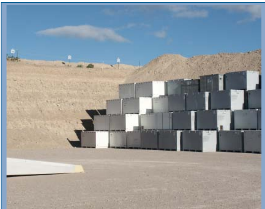
Low-level waste boxes are methodically stacked in a numbered grid system, which aids in waste tracking.
