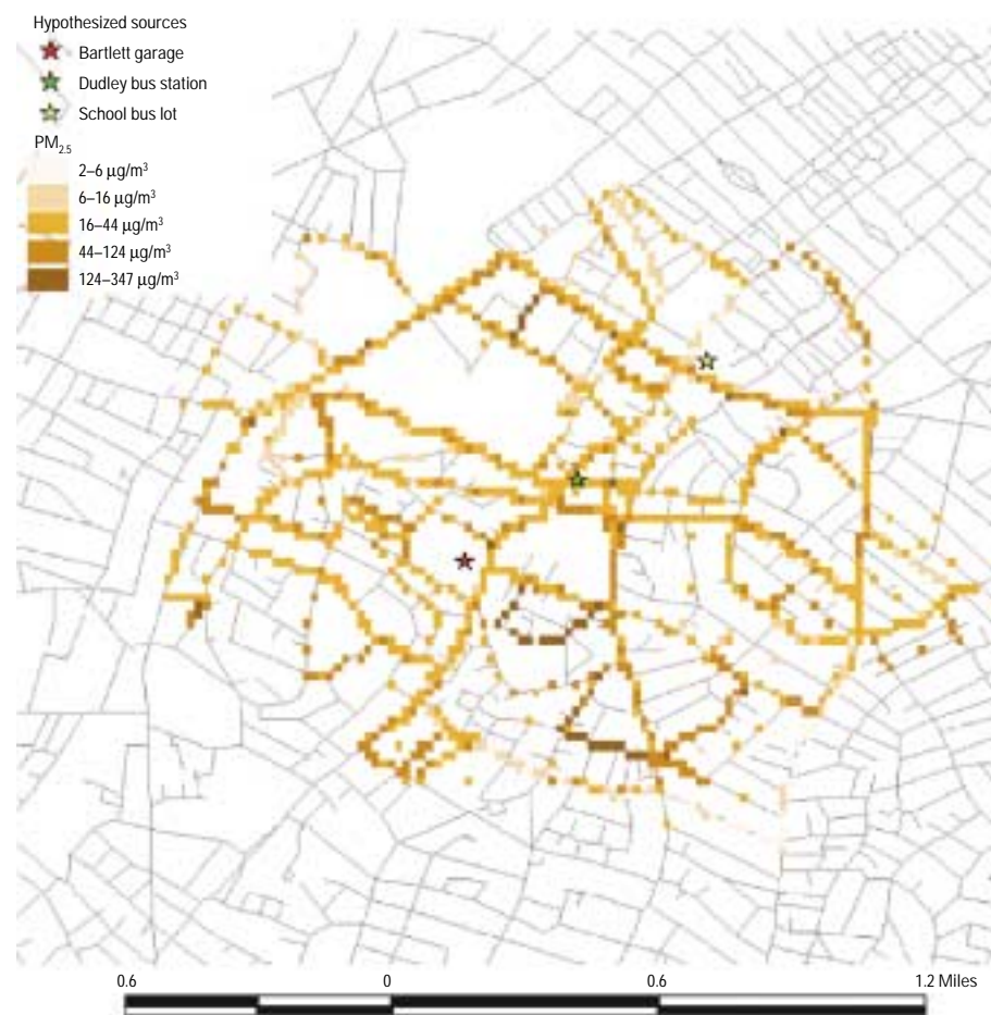
Figure 5. GIS representation of cell-averaged, 1-min average PM_{2.5} concentrations near Dudley Square, derived from mobile DustTrak monitoring in July/August 1999 ( \mu\text{g}/\text{m}^3 ).
