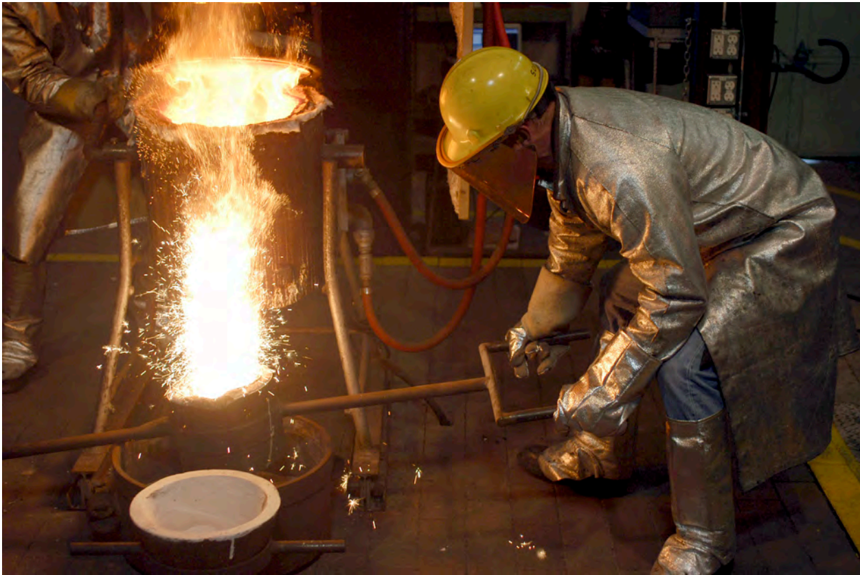
NETL researchers pour molten metal from a bench-scale electric arc furnace during direct smelting tests in cooperative work with Cardero Iron Ore Company, Ltd.
