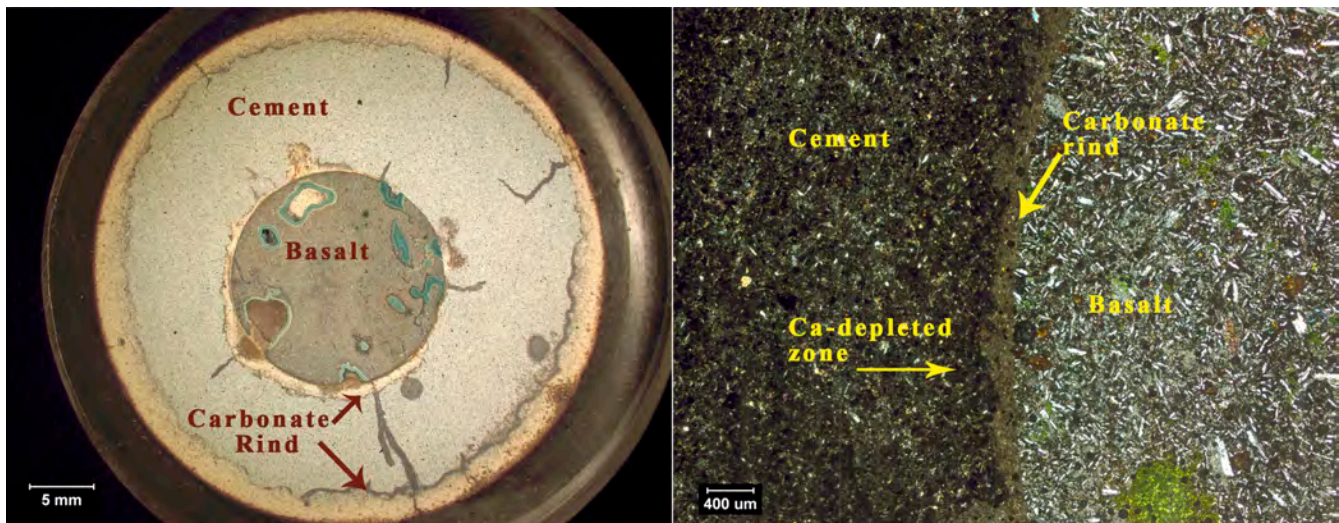
Shown at left is a basalt core within cement at low magnification showing the well cement/rock interface. The photo on the right is a thin section, transmitted light photomicrograph showing the interface between basalt and cement.
