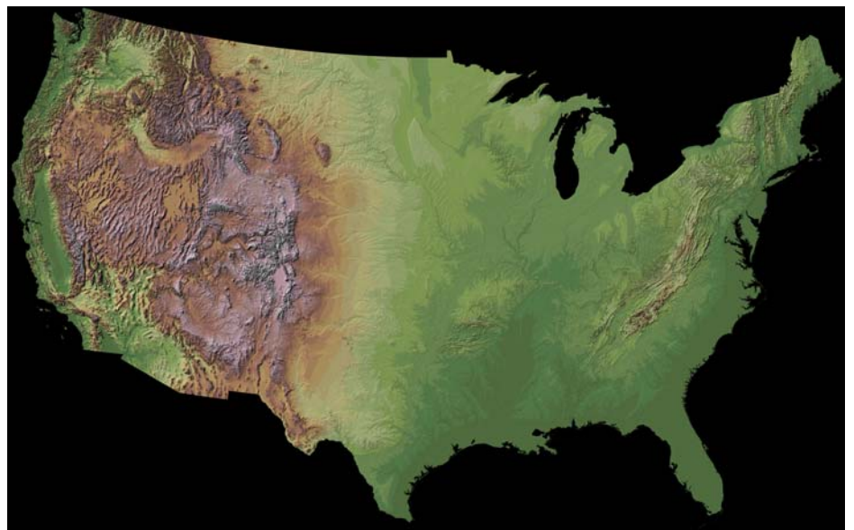
A shaded relief representation of the conterminous United States part of the National Elevation Dataset (NED). Elevation is shown as a range of colors, from dark green for low elevations to white for high elevations.
