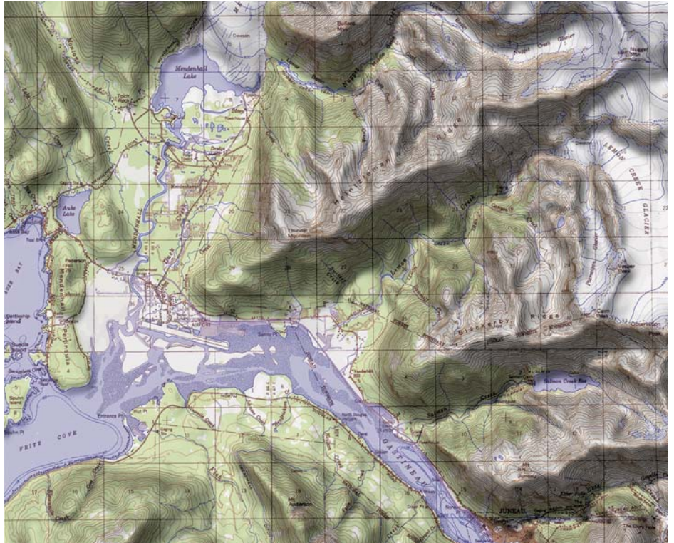
Shaded relief generated from raster elevation data effectively portrays the land surface, shown here in combination with the topographic map content from the USGS digital raster graphic of Juneau, Alaska.
