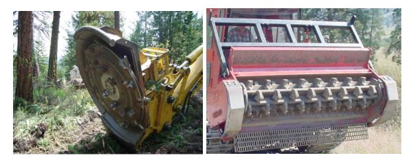
Figure 2. Examples of mastication heads. Vertical shaft (left photo) and horizontal shaft (right photo).
