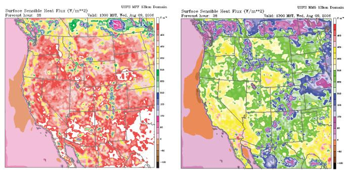
Left image shows daytime fields of sensible heat flux predicted by the new model MFF. Right image shows predictions made by the previous version of MM5 area, both for 13:00 MST on August 9, 2006.
