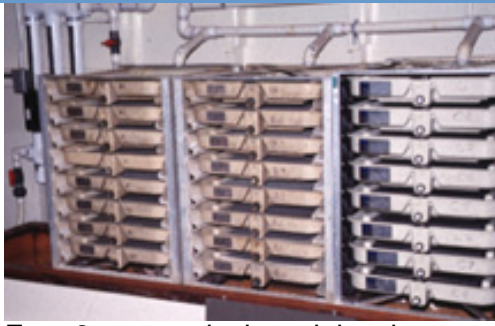
Four 8 tray vertical stack incubators UV Disinfection Temperature Control for Year Round Operation
