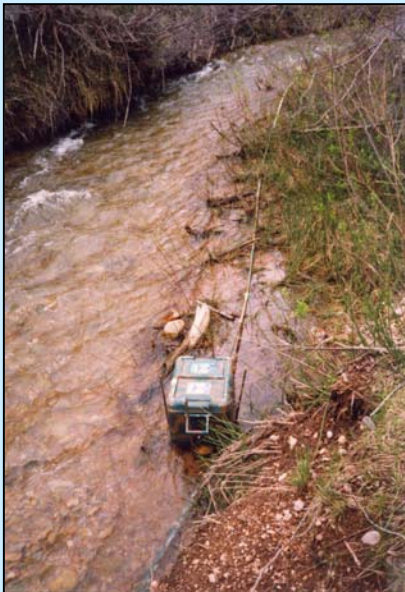
Cooler with 50-feet, 1 inch PVC pipe, gravity flow
