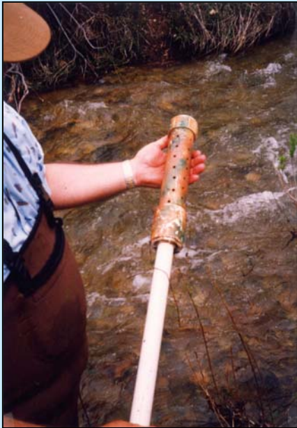
Intake PVC pipe
