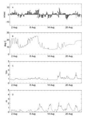
FIG. 3. Weather and water intake data during the deployment. The second tick mark on the horizontal axis is 2 August. A. Wind speed and direction recorded at Muskegon B. Water temperature at the Muskegon water intake. C. Beam attenuation coefficient at the water intake. D. significant wave heights at NDBC buoy 45007.
