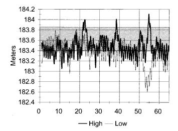
FIG. 10. Lake Superior levels produced by stochastically-generated series of net basin supplies. The experimental net basin supplies were developed based on present climate to provide extreme highs and lows for testing future models. This shows the levels produced by the segment with the highest supplies and the one with the lowest supplies.
