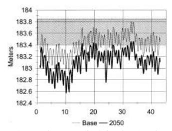
FIG. 9. Lake Superior levels based on Canadian Climate Centre model, CGCM1. The comparison of Base (1961 to 1990) with 2050 (2030 to 2071) indicates a drop in lake levels of approximately 0.3 meters due to greatly increased evaporation caused by warmer air temperatures.
