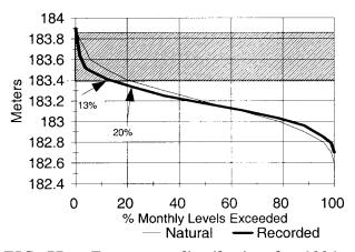
FIG. 7B. Frequency distribution for 1921 to 1972; regulation based on Superior only. When regulation was based on Superior levels only, high levels were reduced by 7%.
