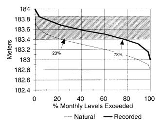
FIG. 7C. Frequency distribution for 1973 to 1999, regulation based on balancing. During recent years when regulation of Lake Superior was based on balancing storage between Superior and Michigan-Huron, regulation more than tripled the occurrence of high levels on Lake Superior. This period also included some very high supplies.
