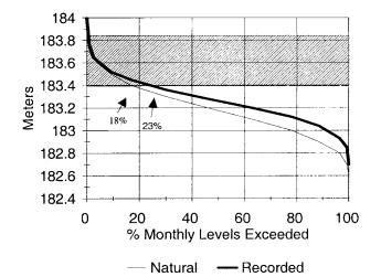
FIG. 7A. Frequency distribution for 1921 to 1999, the entire period of regulation. Regulation of Lake Superior has increased the occurrence of high lake levels by 5%.
