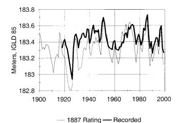
FIG. 11. Comparison of recorded levels with "natural" (1887 Rating) levels for Lake Superior. Regulation appears to have prevented (by at least 10 cm) even lower levels in the 1920s and 1960s. This also shows that regulation increased the peak high levels in the 1980s by over 10 cm.
