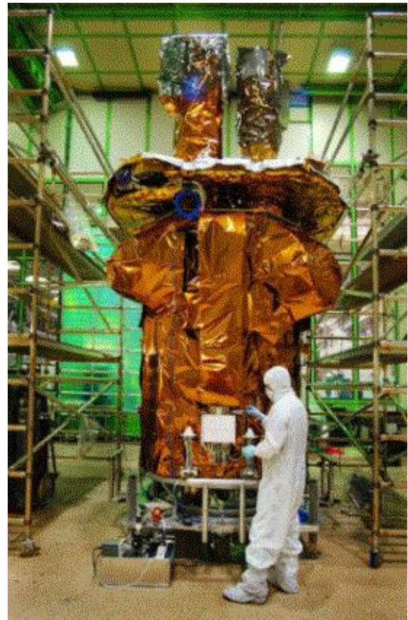
Fig. 5: Swift observatory with Narrow Field Instruments installed. The XRT is the left-hand telescope tube. The white box to the left of the person is the XRT electronics.
