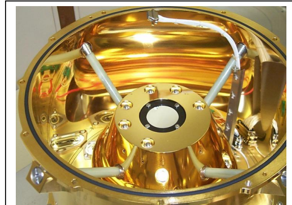
Fig. 16: Interior of the FPCA, showing the lower half of the camera. The circular UV/optical blocking filter is mounted at the top of the lower proton shield, which is mechanically supported by four fiberglass struts. The black ring around the filter is the filter frame, which defines the instrument field of view. The sun shutter assembly mounts immediately above the filter.
