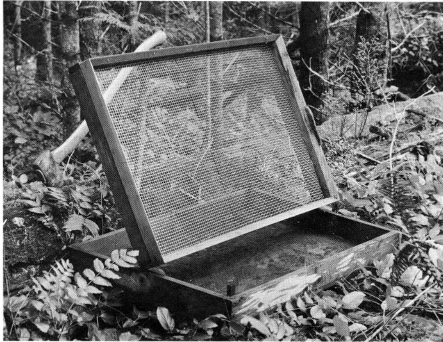
FIG. 2. Seed trap used in the study with top raised for better viewing. (In use, the top rests flat on the bottom portion and is held in place by the pegs at diagonally opposite corners.)
