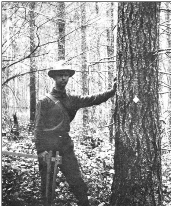
In the early days of the permanent study plot program, large calipers were used to measure tree diameter.
