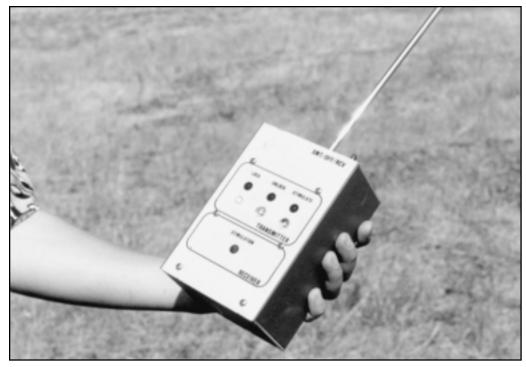
Figure 5—A hand-held unit enables us to lock, unlock, and stimulate eartags and to test the signal from the transmitter.
