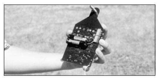
Figure 4—The prototype eartag is powered by two AAA batteries. Electrical stimulation is provided by electrodes on the nylon insulator post at the top of the eartag, which is inserted through an existing hole in the ear of the animal.
