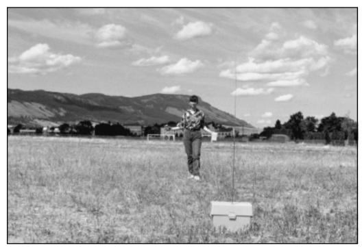
Figure 2—A transmitter housed in a plastic battery case emits a continuous coded signal. Signal distance is determined by approaching the transmitter with an electronic eartag and listening for the audio warning.
