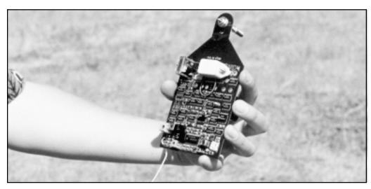
Figure 3—The prototype electronic eartag is 3 inches wide by 6 inches long and weighs about 4 ounces.
