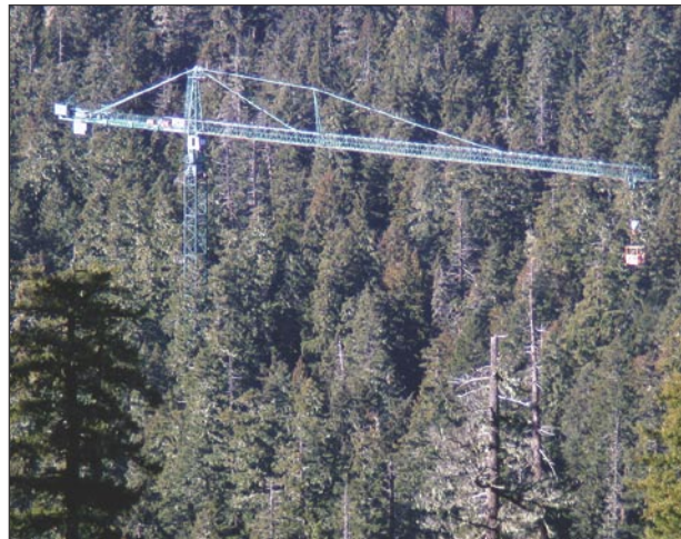
The 250-foot-tall canopy crane gives scientists access to nearly 6 acres of old-growth canopy, making a whole new view of the forest possible. The crane and area around it are closed to the general public owing to safety concerns.
