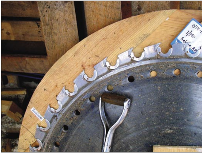
Circular saws cut much wider kerfs than bandsaws. Some wood is lost as sawdust.
