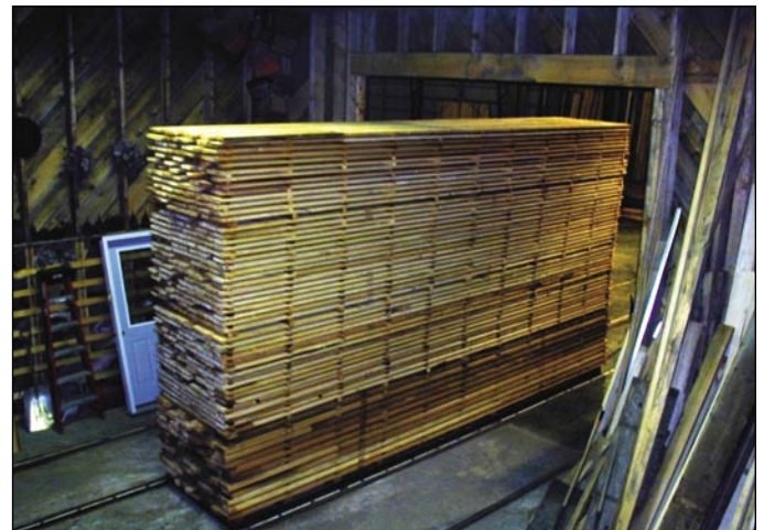
For small sawmills, adding a dry kiln is one way to increase product value. Kiln-dried lumber must be grade stamped, certifying its moisture content, to get the full value premium. Wood residues at sawmills can be used as the energy source to heat kilns.
