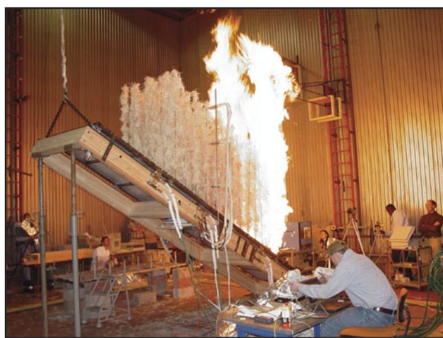
Researchers use controlled experiments at the Fire Sciences Laboratory in Missoula, Montana, to examine heat transfer mechanisms involved in extreme fire behavior.
