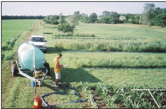
Rain simulation studies help scientists and managers understand how buffer composition and width can impact water quality in buffers over time.
