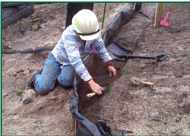
This researcher is scraping out sediment accumulated behind a silt fence to estimate soil erosion.
