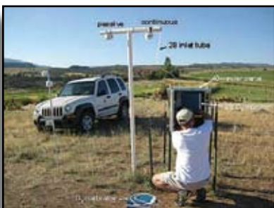
Remote battery powered ozone monitoring station near Silt, Colorado.
