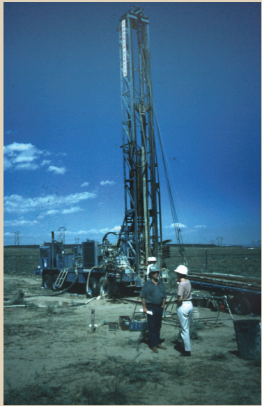
A USGS drilling rig collecting core at the 98th Street well.
