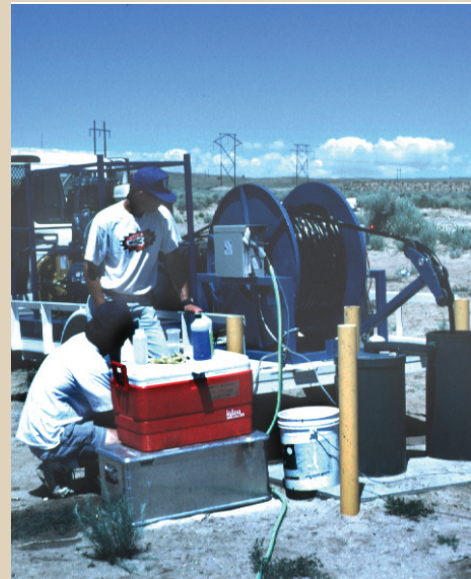
Ground-water sampling at the 98th Street well. Because monitoring wells typically do not contain pumps, a portable sampling pump must be lowered into the well.
