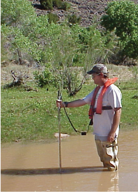
A USGS technician measures flow in the Jemez River below Jemez Dam. Such measurements are critical to understanding ground-water/surface-water interaction.
