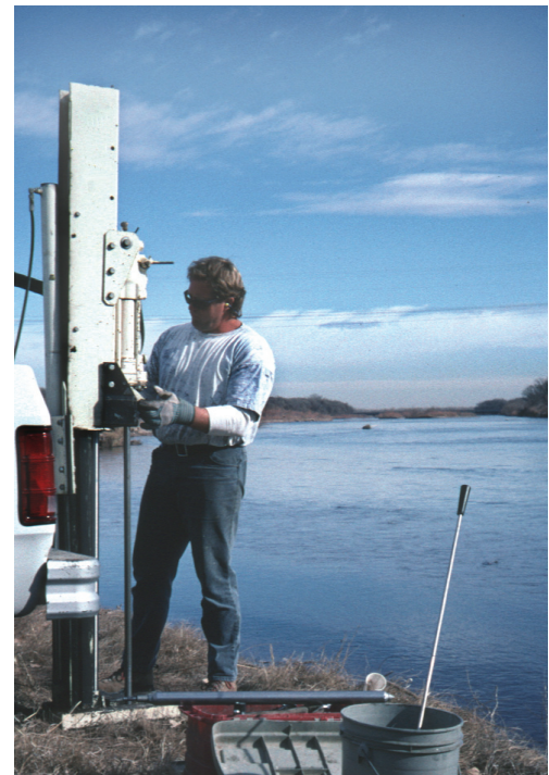
A small truck-mounted soil-probing machine used in the Middle Rio Grande Basin to sample shallow ground water. The size and portability of this unit allow for the collection of more data with less disturbance.
