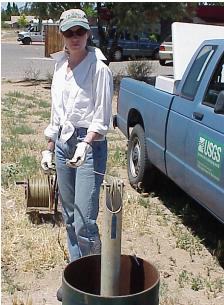
A USGS hydrologist collecting ground-water levels at the Sierra Vista monitoring well. Frequent and consistent measurements of ground-water levels are crucial for understanding the aquifer system and tracking water-level declines.
