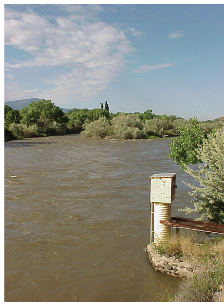
The USGS streamflow-gaging station on the Rio Grande at San Felipe. Such gaging stations provide critical streamflow data for water budgets and water management.
