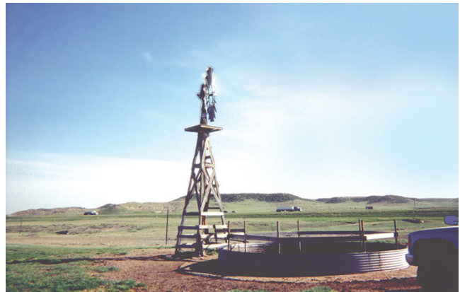
Windmill-powered well and livestock-watering tank in Platte County, Wyoming. (Photograph courtesy of J.P. Mason, U.S. Geological Survey.)
