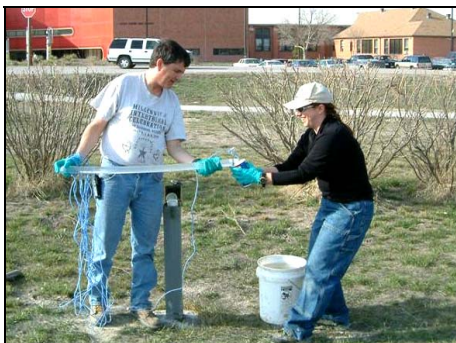
EPA staff conducting LUST sampling with the UST/LUST Coordinator for the Oglala Sioux Tribe (Pine Ridge, SD)
