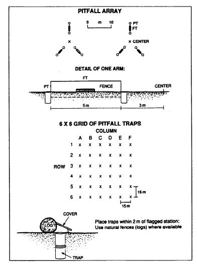
Figure 3—Designs for arrangements of pitfall traps either with or without drift fences. PT = pitfall trap, FT = funnel trap.
