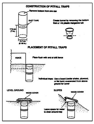
Figure 4-Construction and placement of a pitfall trap.
