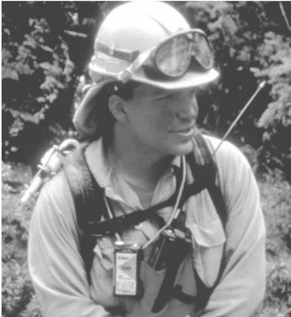
Figure 6—Datalogger in the breathing zone.
