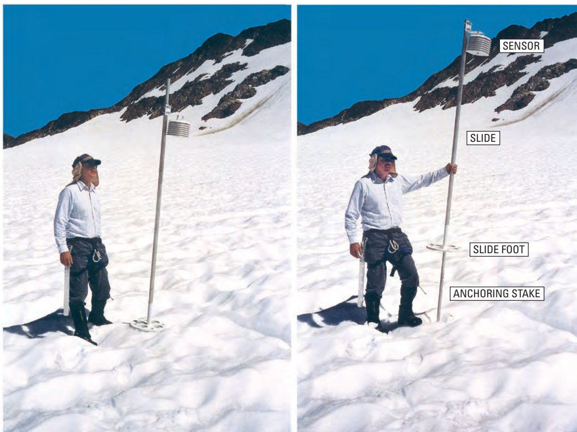
Figure 3. Self-adjusting mount for an air-temperature sensor over a glacier.
