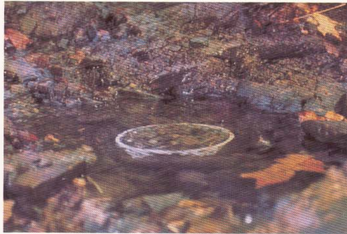
Figure 4-1a,b. Rock basket colonization sampler used to characterize aquatic macroinvertebrate communities.
