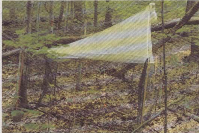
Figure 8-1. Townes-style Malaise trap used to collect adult insects, Fernow Experimental Forest.
